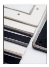
KC Shielding - Knitted mesh over an elastomer core bonded to a nonconductive material carrier to provide an environmental seal - usually fitted with a self-adhesive strip to aid mounting (also known as twinstrip)
