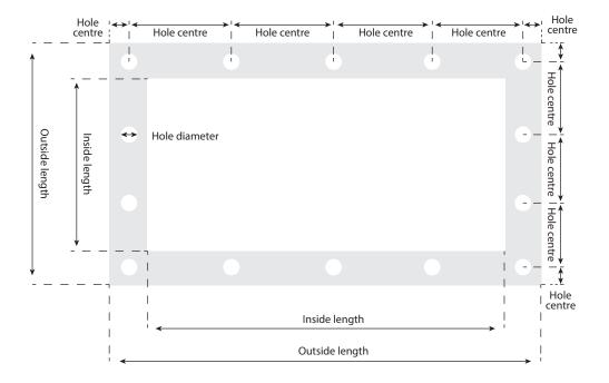
Usually square or rectangular in shape, picture frame gaskets will require both outside and inside measurements (which can be achieved with a tape measure). These types of gaskets will likely have bolt holes around the frame and often of consistent diameter and spacing (although this may not always be the case, so it is best to check). The above image provides full details on all measurements required for picture frame gaskets.
