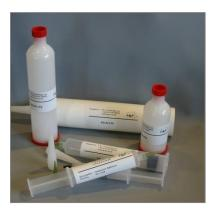
P & P Technology AS-N is a single component electrically conductive adhesive comprising of silicone resin filled with conductive nickel coated graphite particles. It cures on exposure to air at room temperature to form an electrically conductive flexible silicone elastomer. Once cured it adheres strongly to a wide range substrates.
