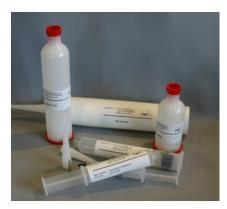
P & P Technology AS-H is a single component electrically conductive adhesive comprising of silicone resin filled with conductive silver plated copper particles. It cures on exposure to air at room temperature to form an electrically conductive flexible silicone elastomer. Once cured it adheres strongly to a wide range substrates.
