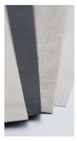
MF Shielding is a range of highly conductive metallised fabrics. They consist of a base material of nylon coated with nickel/copper. The fabrics have excellent conductivity in all directions and exhibit excellent EMI shielding effectiveness. They are very flexible and are ideal for wrapping around core material or for die stamping.
