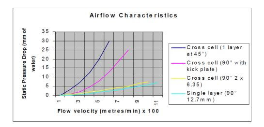
Airflow characteristics applicable to vent types VH AF1, VH AF2, VH AF3 & VH AF4.
