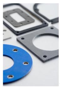
P & P Technology SP, SS, SR, SW & SF ranges of gasket materials consist of Monel, aluminium or phosphor bronze wires embedded into solid silicone, sponge silicone or fluorosilicone with a flame retardant variant also being available.
